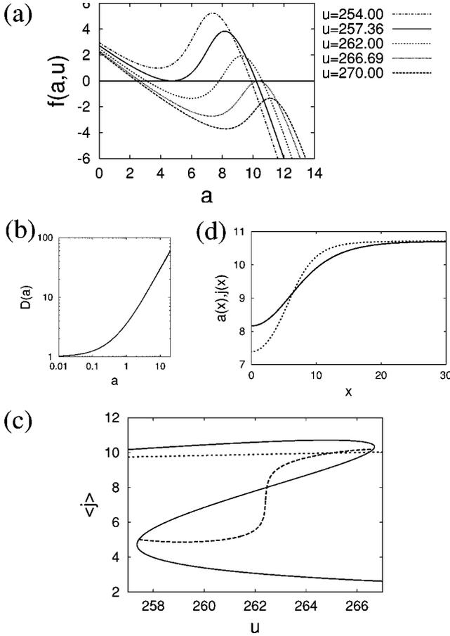
FIG. 2. (a) Nonlinear kinetic function  $f(a,u)$  for different values of voltage  $u$ , (b) diffusion coefficient  $D(a)$  as a function of the electron density  $a$  (double-logarithmic scale), (c) current-voltage characteristic for spatially homogeneous states (solid line) and filamentary states (dashed line) for  $L=30$ ; load line for  $U_0 = -84.2895$ ,  $r = -35$  (dotted line), (d) spatial profile of a half filament,  $a(x)$  (solid line) and  $j(x)$  (dotted line) ( $L=30$ ;  $u=265$ ).
